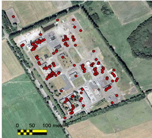
Figure 2. Close-up of point coverage for an underground storage cavern, Germany (PSI data copyright TRE 2005. ERS data copyright ESA 1992-2005. Background image copyright Landesvermessungsamt Nordrhein-Westfalen).
