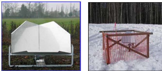
Figure 8. Corner Reflectors: a) ground view of a deployed CR (copyright NPA), b) CR and protective wooden fencing installed at the Canadian site (copyright EBA).
